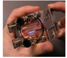
confusion is impossible. The slightly differing spring displacements on both sides cause the pressure to finally concentrate exactly on the processor core ("balanced load"). Now insert the pressure springs into the
