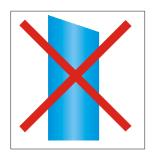
1. Cleanly cut the hose to the desired length. The hose should be cut **evenly** and cleanly **avoiding burs** with a sharp knife or a hose cutter (available in our shop). After each detachment of the hose from a connector the first two centimeters have to be cut off to guarantee a secure operation.
